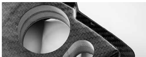
Machining processes compared: dry (left), rhenus special coolants (right)
